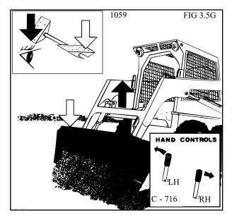
To level the ground; raise the lift arms and tilt the bucket down by pressing on the toe of the bucket pedal (Fig. 3.5H). Push firmly on the toe of the lift arm pedal to lock the lift arms in float position. The weight of the lift arms and bucket will hold the bucket on the ground. Drive backward to level material.
