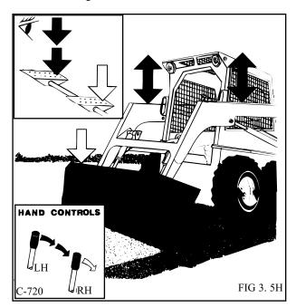
To fill a hole (Fig. 3. 5I) drive the loader slowly with the bucket low, up to the hole. As the bucket passes the edge of the hole, push on the toe of the bucket pedal to dump the bucket. When necessary raise the lift arms to empty the bucket.
