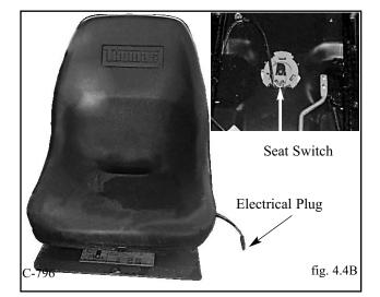
The seat and seat plate can be removed to provide access to the controls, hydraulic and hydrostatic components. To remove the seat assembly, remove the fasteners located at the front of the seat. *Disconnect the electrical plug!!* Lift the seat assembly out of the machine. When installing the seat, be sure the seat plate locks are in place at the rear (Fig. 4. 4B).
