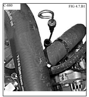
Keep the oil level between the full and low mark on the dipstick (Fig. 4. 7B2). Do not fill above the full mark and use only appropriat oil (See Section 5 for specifications).
