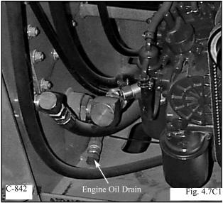
Remove the oil filter (Fig. 4. 7C2). Clean the filter housing surface. Put clean oil on the seal of the new filter and install the filter hand tight. Replace the oil drain plug. Remove the filler cap and add appropriate engine oil (See Section 5 for specifications). Start the engine and run for 5 minutes. Stop the engine and check for leaks at the filter. Recheck the oil level and add oil until the level is at the top mark on the dipstick.
