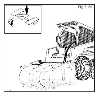
auxiliary pedal until the pedal locks in detent position. When the auxiliary circuit is not in use return the auxiliary pedal to neutral position otherwise starting the loader may be difficult or impossible.
